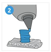
In the center of your square, begin to build up the base of the tower by **tightly coiling the plastic as it extrudes.**
